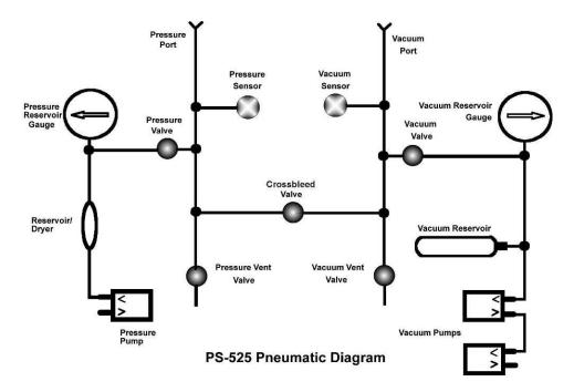
When the operator wishes to simulate an altitude, the Crossbleed, Vacuum, and Vacuum Vent valves are gently closed. The vacuum pump is then energized until sufficient vacuum is in the reservoir, as indicated on the Vacuum Reservoir Gauge. How much vacuum will be needed depends on the desired altitude, and is also affected by how long
